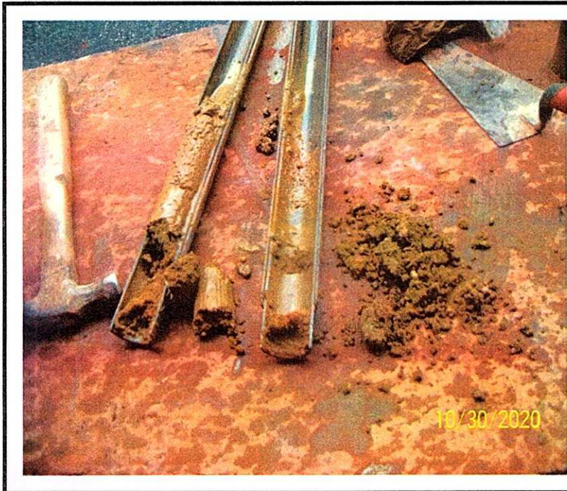
Sample recovery from split spoon samplers
