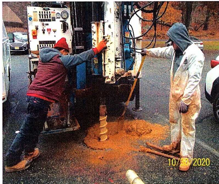
Sample procurement using split spoon samplers and augurs
