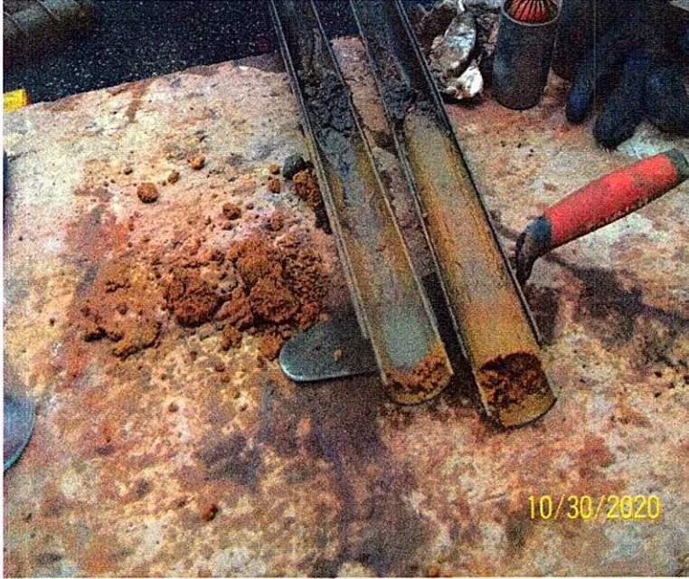
Sample recovery from split spoon samplers
